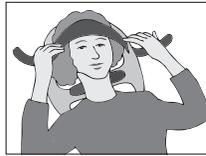
(see illustrations) *Note: For smaller heads and shorter necks locate Comfort Visor™ in forward slots. For larger size locate Comfort Visor™ in back slots.*
