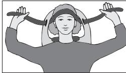
4. Hold back of unit down with tips of index fingers or thumbs and further tighten Comfort Visor™ if necessary. (see illustration above)
